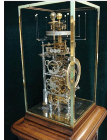
**Photo 8: Paul Pouvillon, France, c. 1930, an extraordinary astronomical clock with more than 44 various indications. Considered the most complicated clock built for its size, 20 inches high.**
