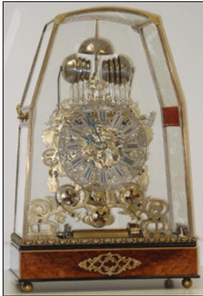
**Photo 6: Smith of Clerkenwell, England, c. 1850, ivy leaf design. Complex quarter-striking clock with four-tune music box tripped automatically six times per day.**
