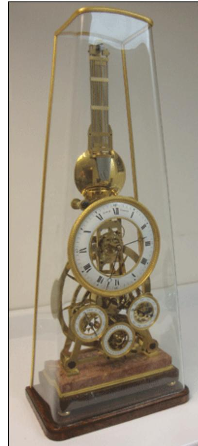
**Photo 7: Henry Lepaute, France, c. 1830, inverted pendulum design with day, date and month calendar, 29 inches high.**
