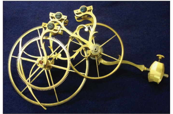
Figure 16, above. One of the two time train Wagner remontoire.
