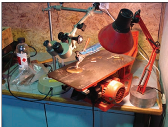
Figure 1. Jeweler's saw with binoculars to cut all flat stock.
