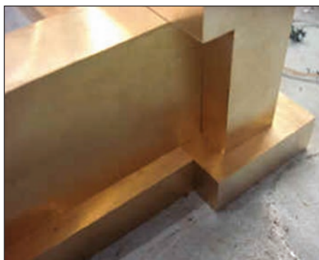
Figure 19, top. Frame and molding detail fabricated in wood model.
