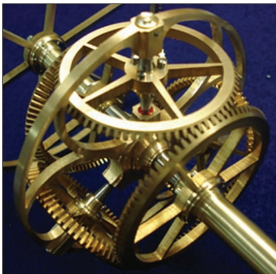
Figure 29. Differential drive for dual time train remontoire.
