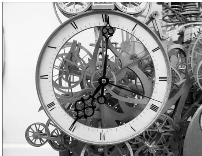
Figure 10. Mean solar (clock time) dial. The sun hand indicates the time as would be read on a sun dial. The difference in minutes between it and the clock time minute hand is the equation of time.
