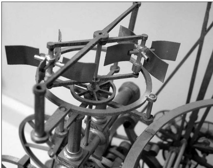
Figure 3. One of a pair of compound epicyclic flies mediating the two remontoire.
