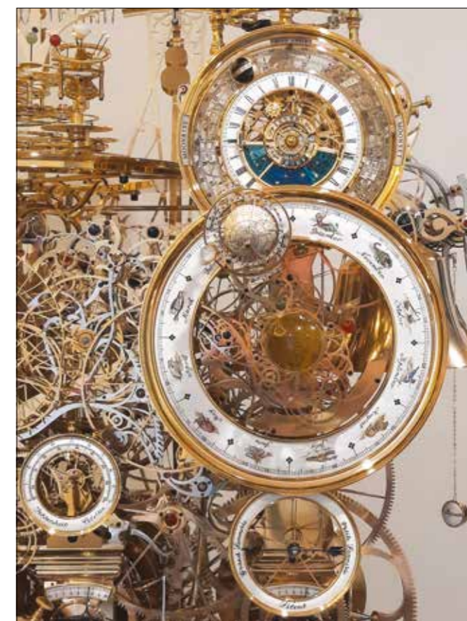
Figure 16A. Right side, Sun and Moon module, tellurion, strike selector, thermometer.
