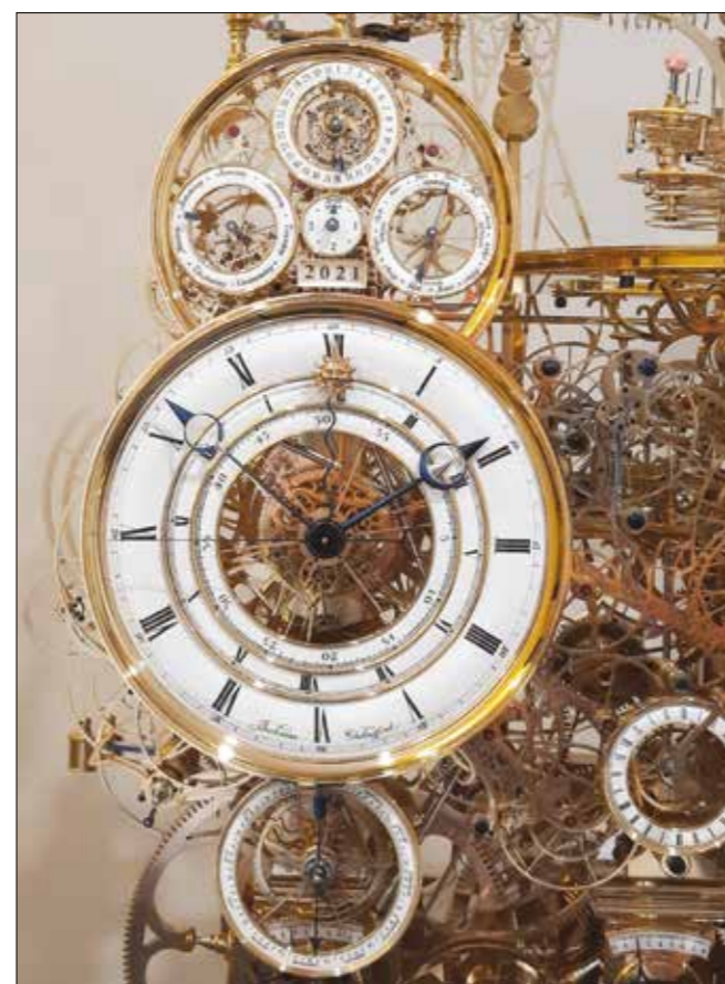
Figure 15. Left side, calendar, mean, sidereal, equation time.
