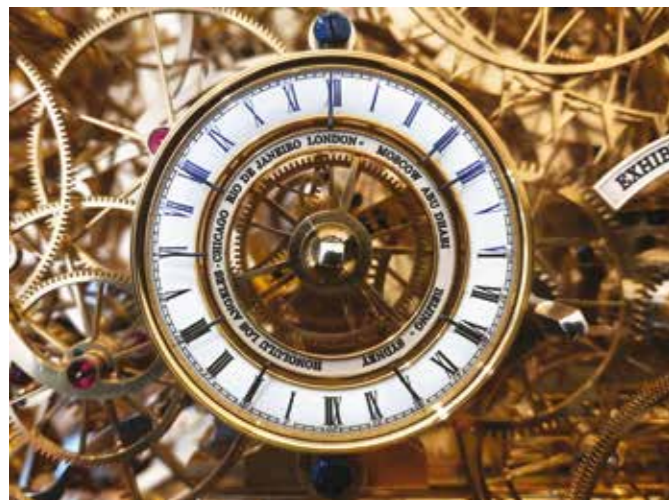
Figure 16B. International time dial and demonstration drive.
