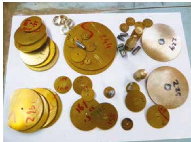
Figure 26. 54 wheel blanks, pinions plus miscellaneous parts.
