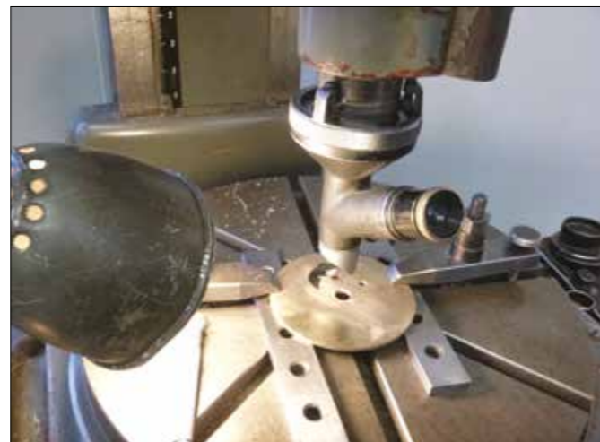
Figure 27. Setting jewel pivots in the jig borer with the microscope.
