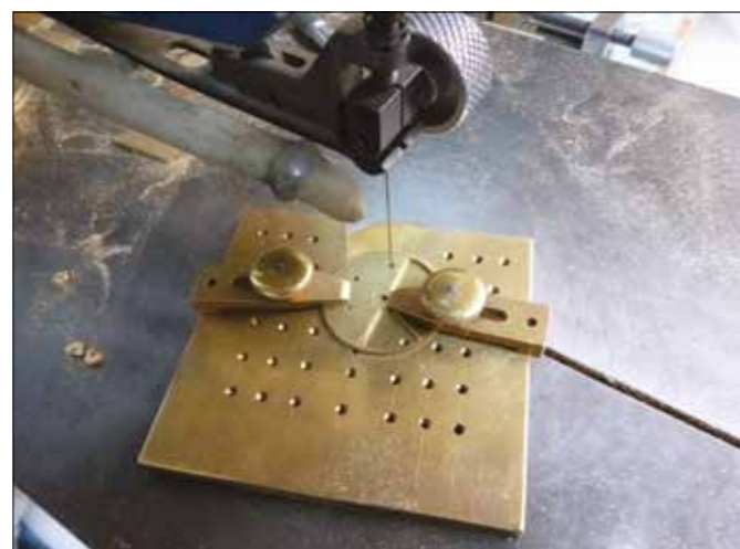
Figure 29. The crossing-out process on a scroll saw.
