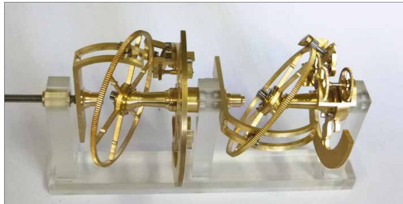
Figure 32. The Projection differential (left) and Great Anomaly differential (right), slaved together to produce a combined output.
