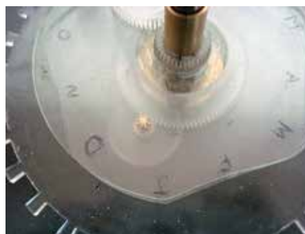
Figure 78. Cam with flat cut for February.
