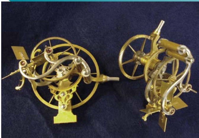
Figure 14. Two left- and right-hand strike train governors.
