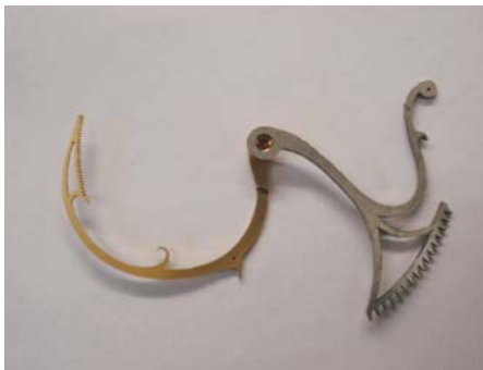
Figure 24. Completed quarter strike rack before finishing.
