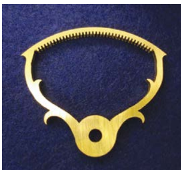
Figure 27. Interior toothed sector gear with ivy spur design.
