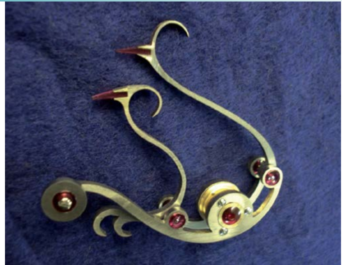
Figure 32. Bird analog seesaw quarter rack advancer.
