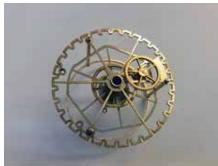
Figure 95. Delicately cut crenulated index wheel and cams.
