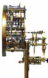
Figure 131. Right-side view of calendar complication.
