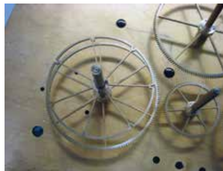
Figure 102. Stepper wheel mounted above its drive wheel.
