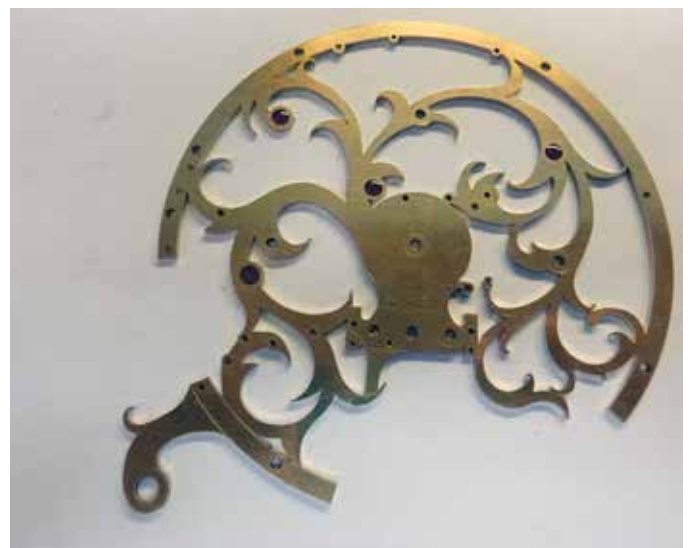
Figure 125. Rear frame fretted, displaying organic ivy design.
