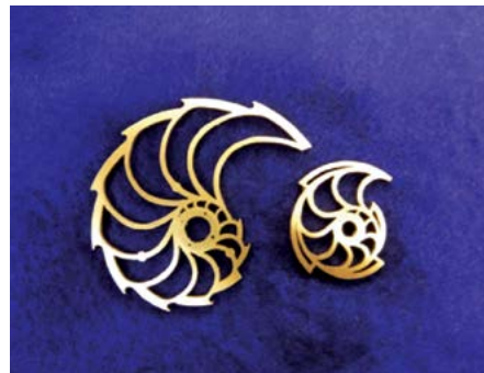
Figure 26. Hour and quarter snails as nautilus shell cross sections.
