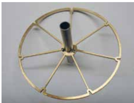
Figure 101. Stepper wheel for day of the week.
