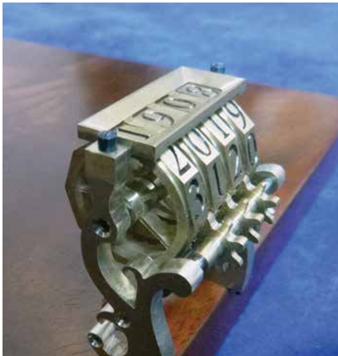
Figure 106. Digital year readout.
