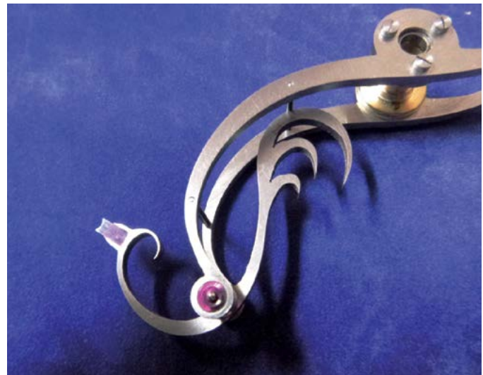
Figure 33. Bird analog bell hammer actuator.
