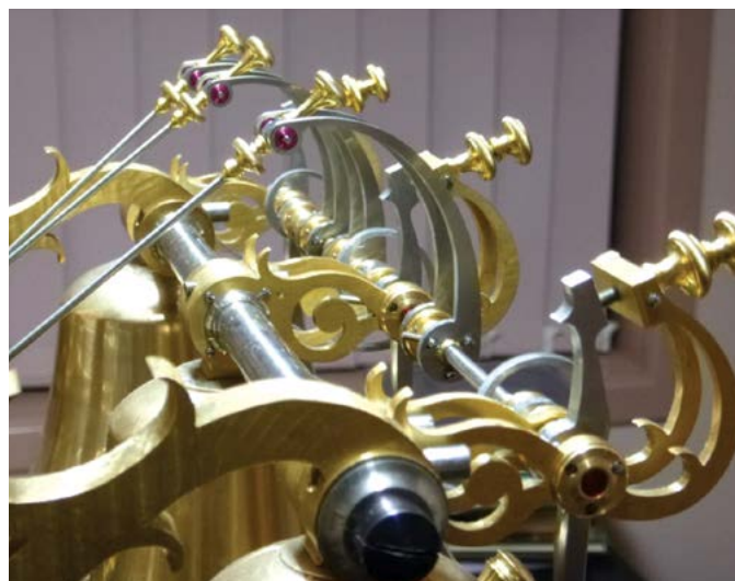
Figure 43. Hammer adjustment controls with decorative knurls.
