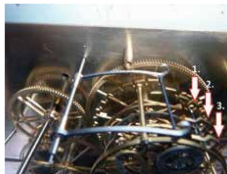
Figure 104. Arrows point to locking detents for each dial's readout.
