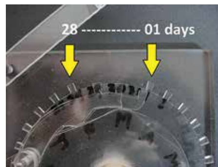
Figure 76. The surprise pieces for Days 29, 30 and 31 between the two arrows are lowered, giving February 28 days.
