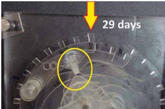
Figure 87. Cam correcting every 400 years. Arrow points to cam.
