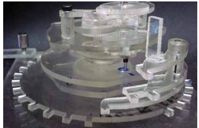
Figure 90. Three-quarter view of perpetual calendar module.
