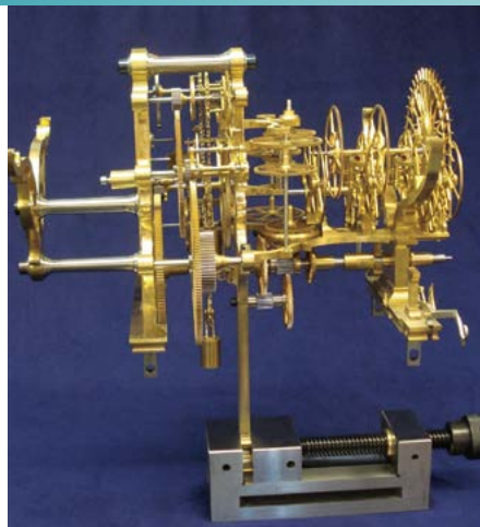
Figure 5. Side view of center module, celestial train, and escapement with Robin remontoire.
