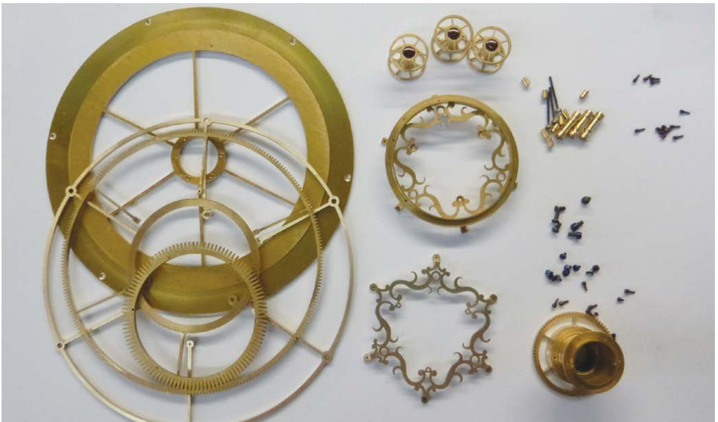
Figure 59. Sixty-eight parts in the sidereal hour and minute concentric ring drives.
