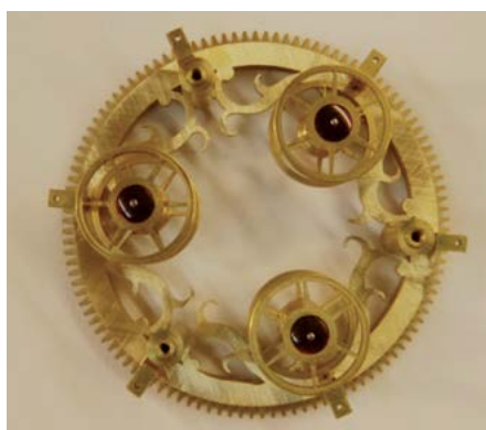
Figure 54. Three roller wheels added to rear frame.
