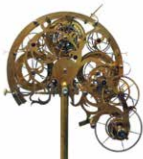
Figure 133. Rear view of calendar complication.
