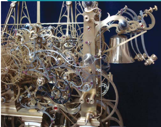
Figure 40. Front view of strike control levers installed.
