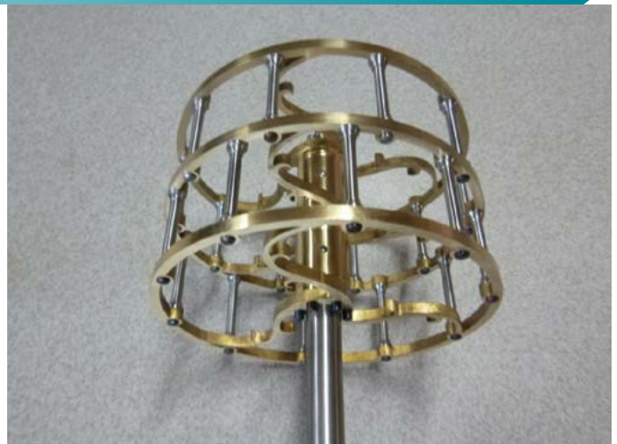
Figure 30. Quarter strike cam carousel.
