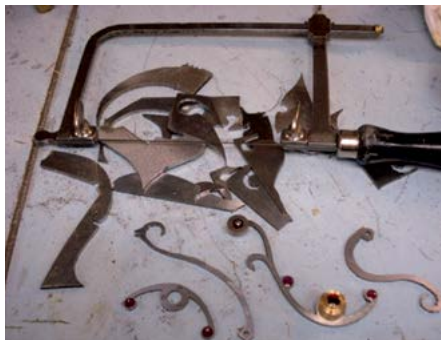
Figure 25. Hand fretsaw used to cut racks and other parts.
