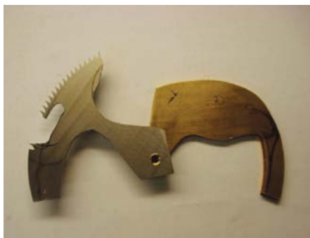
Figure 22. Quarter rack in metal.
