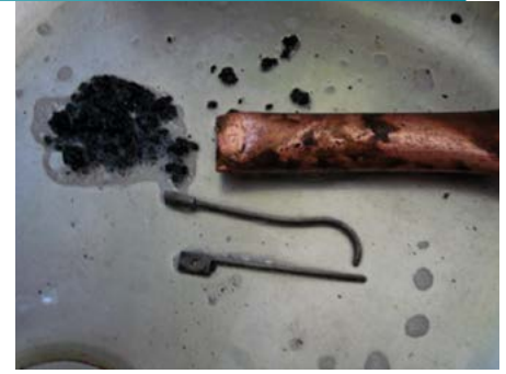
Figure 38. Water used to harden springs in copper envelope.
