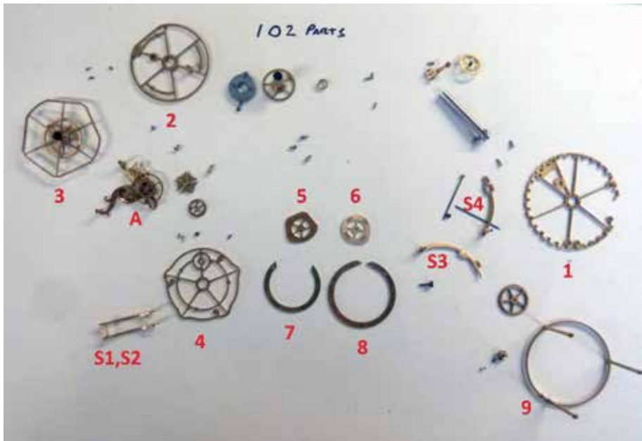
Figure 96. Components of the perpetual module. The numbers and the letter as well as their descriptions of the main components are as follow:
