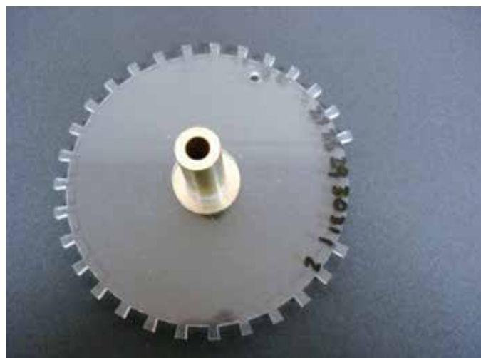
Figure 68. Daily index wheel for days 1-28.
