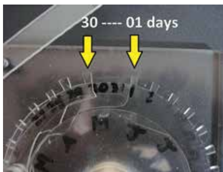
Figure 75. The surprise piece for Day 31 between the two arrows is lowered, giving a 30-day month.
