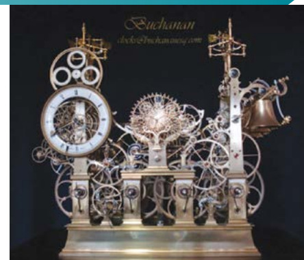
Figure 9. Celestial train mounted to base frame.
