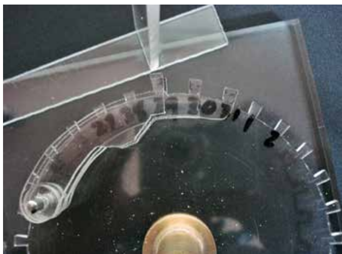
Figure 71. Surprise pieces over index wheel.
