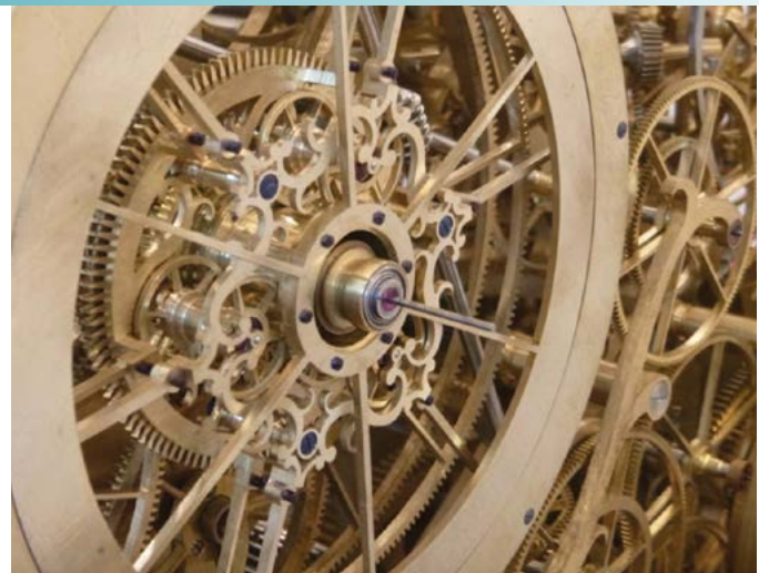
Figure 60. Completed sidereal drive unit.
