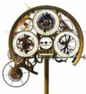
Figure 130. Front view of calendar complication.
