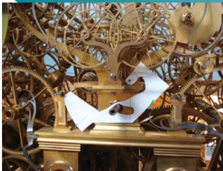
Figure 18. Paper cutout of hour rack.
