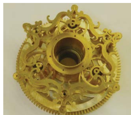
Figure 55. Center hub and rollers set between the frames.
