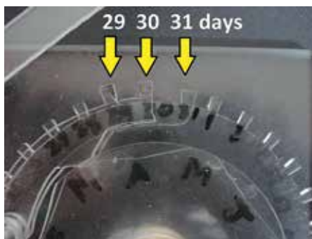
Figure 74. Arrows point to three raised surprise pieces, creating a 31-day month.
