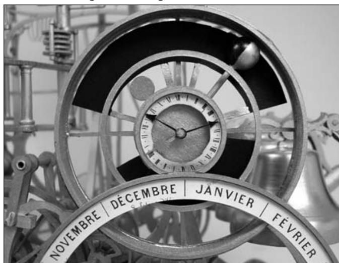
Figure 17, right. Dials with moveable shutters to indicate sun and moon rising and setting.
