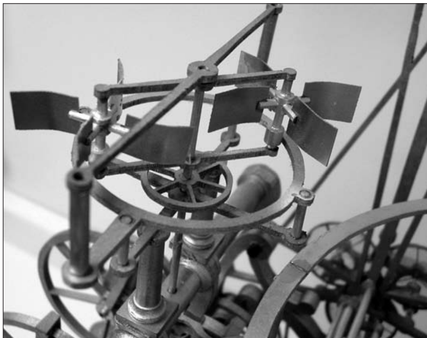
Figure 3. One of a pair of compound epicyclical flies mediating the two remontoire.
